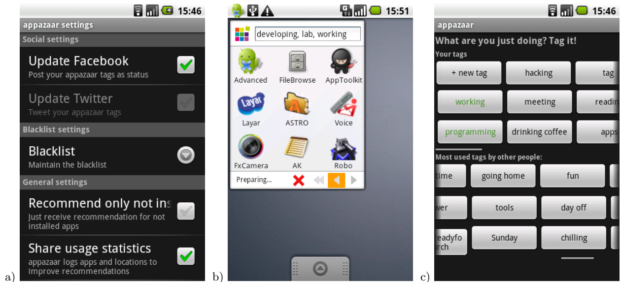
Figure 2: Screenshots of the prototype: a) settings to control the logging, b) access of recommendations within a widget, and c) input of contextual keywords.
